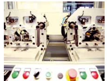
Lens Crimping Assembly 车前大灯组装
