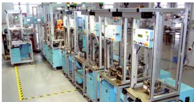
Ignition Coil Assembly Line 高压点火线圈组装产线
