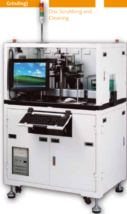
Disc Hub Assembly Assemble disc to hub with an adhesive tape in clean room environment and high precision.
