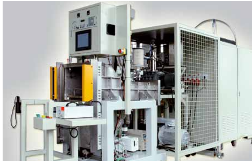
Single chamber with helium recovery system recycling up to 90% of tracer gas
